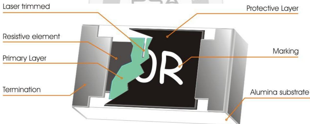
Fig 1. Construction of Chip-R
